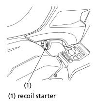
The recoil starter (1) is used to start the engine when the battery is low. See Using the Recoil Starter (Canada only) page 88.
