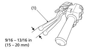
(1) rear brake lever/parking brake lever
