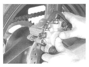
Remove the pad pin plug and loosen the pad pin.
