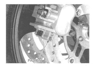
Install and tighten the pad pins.
