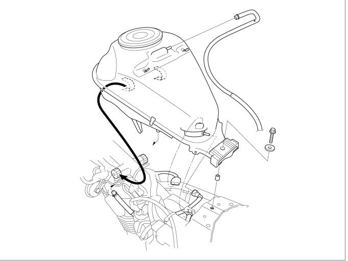
• Quick connect fitting (fuel pump side) →2-2
