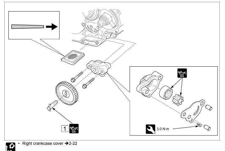
• 1 Align with the cutouts of the oil pump drive shaft and inner rotor.
