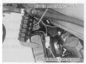
Remove the radiator from the upper and lower brackets by moving it to the left, then move the radiator/oil cooler forward as an assembly.
