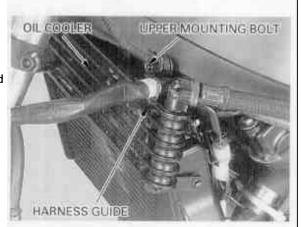
Disconnect the fan motor sub-harness 2P (Natural) connector.
