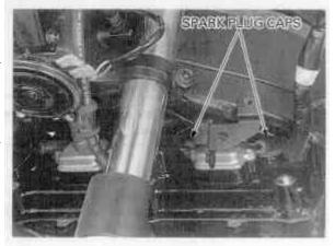
Remove the spark plug using a equipped spark plug wrench or an equivalent.
