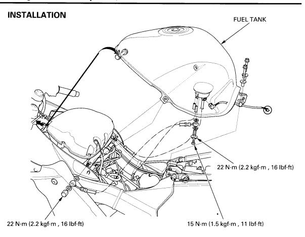
Connect the fuel tube to the fuel pump with new sealing washers.
