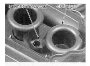
Install and tighten the air funnel/air cleaner housing mounting screws.
