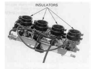
Apply oil to the insulator inside surfaces for ease of throttle body installation.
