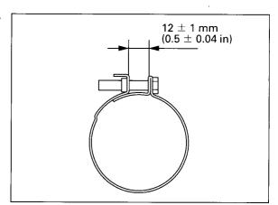
Connect the water tubes to the first idle wax unit, tighten the clamp screw securely.
