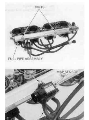
Install the MAP sensor aligning it boss with the hole in the fuel pipe.
