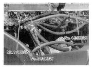
Remove the plugs and connect the PAIR air suction hoses to the reed valve covers.
