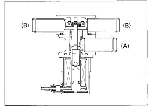
Check the resistance between the terminals of the PAIR solenoid valve.
