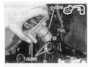
Align the mounting bolt holes in the water pump and crankcase and make sure the water pump is securely installed.
