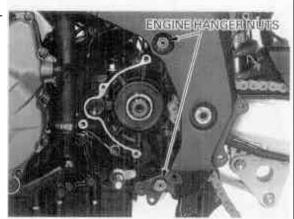
Loosen the rear/upper engine hanger adjusting bolt lock nut while holding the adjusting bolt using the special tool.
