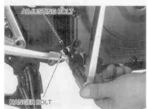
Tighten the rear/upper engine hanger adjusting bolt to the specified torque.
