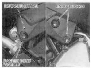
Tighten the rear/lower engine hanger adjusting bolt to the specified torque.
