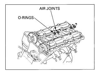
Install the cylinder head cover onto the cylinder head.
