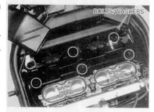
Install the PAIR reed valve covers and tighten the SH bolts to the specified torque.
