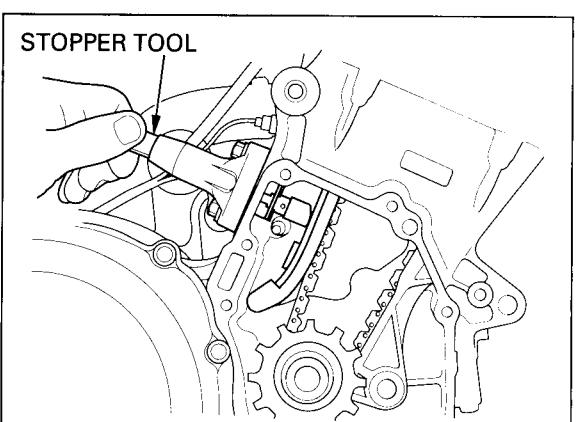
Install a new sealing washer and tighten the sealing bolt securely.
