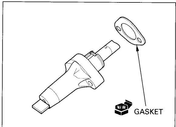
Install the cam chain tensioner lifter into the cylinder block.
