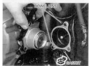
Install and tighten the SH bolts to the specified torque.
