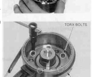
Check the starter driven gear for abnormal wear of damage.
