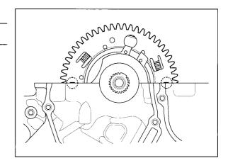
Install a new O-ring into the groove of the front balancer shaft.
