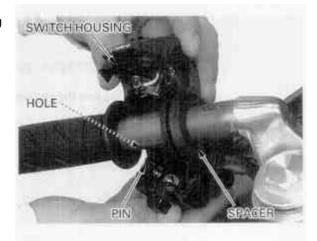
Tighten the forward screw first, then the rear screw.
