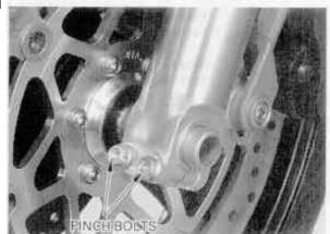
Check the clearance between the brake disc and caliper bracket on each side after installation. The clearance should be at least 0.7 mm (0.03 in).
