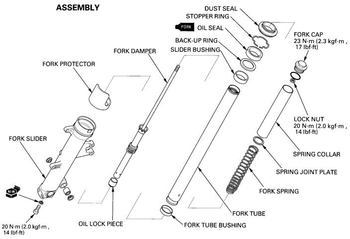
Before assembly, wash all parts with a high flash or non-flammable solvent and wipe them dry.
