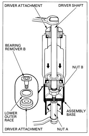
Install a new upper outer race and the ball race remover as shown.
