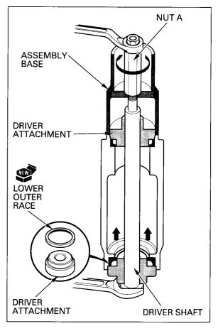
Temporarily install the steering stem nut onto the stem to prevent the threads from being damaged when removing the lower bearing inner race from the stem.
