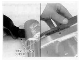
Apply a locking agent to the drive chain slider bolt threads.
