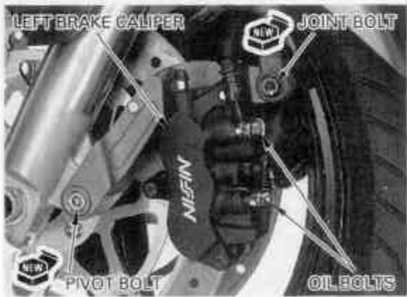
Push the brake hose eyelet to the stopper on the caliper, then tighten the oil bolt to the specified torque.
