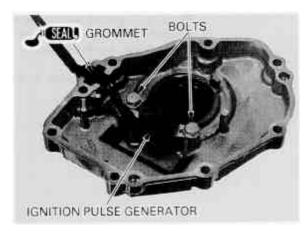
Apply liquid sealant to the mating surface of the crankcase as shown.
