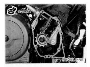
Apply sealant to the threads of the two bolts indicated by " $\triangle$ " mark on the cover. Install the ignition pulse generator rotor cover and
