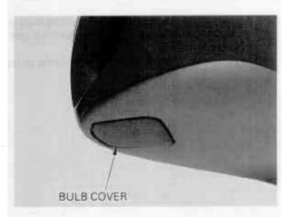
Pull out the position light bulb socket, and replace the bulb with a new one.
