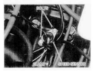
Connect the speed sensor 3P (White) connector.
