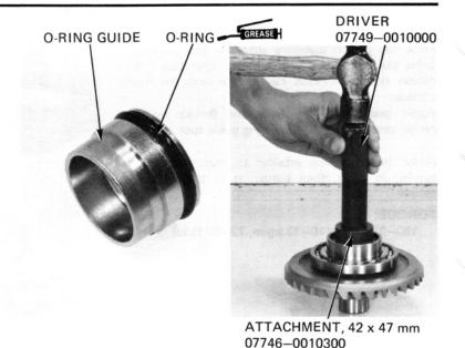
Install the ring gear into the gear case cover. Measure the clearance between the ring gear and the ring gear stop pin with a feeler gauge.
