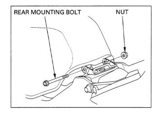
Rear cylinder Raise the rear of the fuel tank and support it with the maintenance bar.
