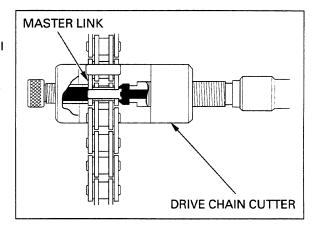
Make sure that the master link pins are staked properly by measuring the diameter of the staked area.
