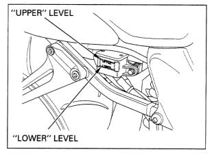
If the level is near the "LOWER" level line, remove the reservoir mounting bolt, reservoir cap, set plate and diaphragm, and fill the reservoir with DOT 4 brake fluid from a sealed container to the upper level line.
