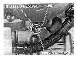
Remove the oil pressure switch and connect an oil pressure gauge attachment and gauge to the pressure switch hole.
