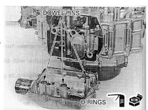
Install the oil pan and cover stays, and tighten the twelve bolts in a crisscross pattern in 2 or 3 steps.
