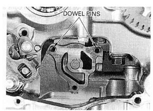
Install the oil pump and tighten the mounting bolts securely.
