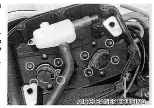
Disconnect the front and rear crankcase breather hoses and air hoses from the air cleaner housing. Remove the air cleaner housing.
