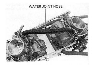
Remove the cotter pins, washers and throttle link.
