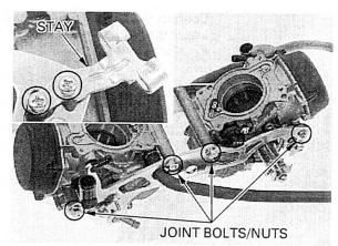
Install the following onto the throttle arm pin: Front carburetor:
