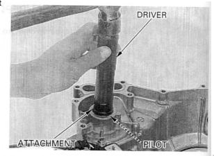
Support the bearing inner race properly and install the water pump shaft until it is seated.
