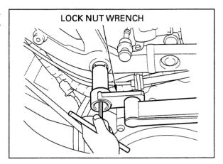
9. Tighten the rear engine hanger nut to the specified torque.
