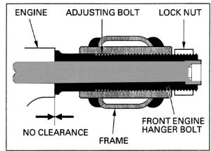
8. Hold the front adjusting bolt with the front engine hanger bolt and tighten the lock nut to the specified torque using the special tool.
