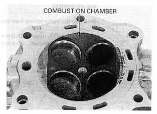
Check the cylinder head for warpage with a straight edge and feeler gauge.
