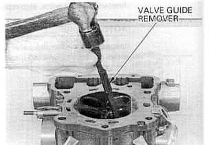
While the cylinder head is still heated, drive new valve guides in the cylinder head from the camshaft side until the exposed height is 14.0-14.2 mm (0.55 -0.56 in).
