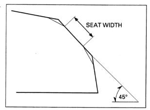
After cutting the seat, apply lapping compound to the valve face, and lap the valve using light pressure.
