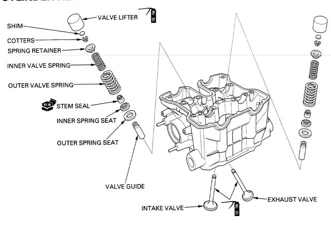
Blow through all oil passages in the cylinder head with compressed air.
