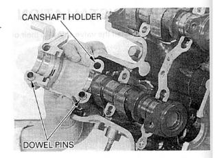
Apply oil to the threads and seating surfaces of the camshaft holder bolts.
