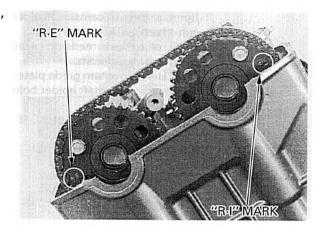
If the timing marks are facing outward, turn the crankshaft counterclockwise 1-1/4 turn (450  $^{\circ}$  ) and align the "FT" mark with the index mark.
